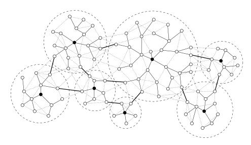
Figure 6.1: A cluster partition of a network: The dashed cycles specify the clusters, cluster leaders are black, the solid edges are the edges of the intracluster trees, and the bold solid edges are the intercluster edges
